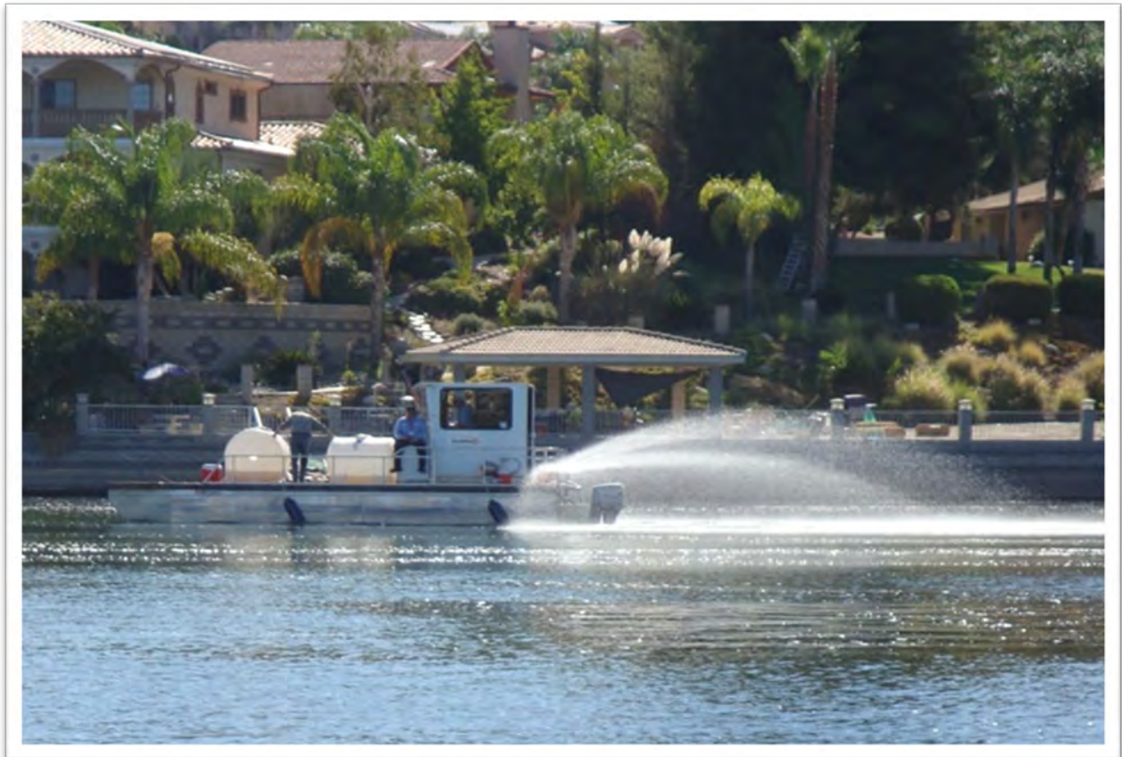
Aquatechnex biologists applying Alum on Canyon Lake
