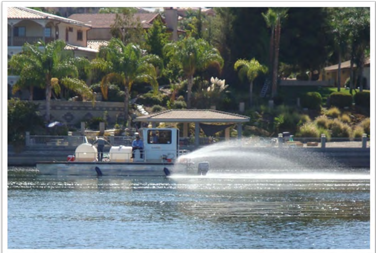
Aquatechnex biologists applying Alum on Canyon Lake
