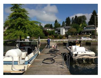
We have a fleet of application vessels for larger open water application of alum. These two vessels can move 8,000 pound on the water, perform precision application and move back quickly to the access site to reload. We can process on tank truck of alum in approximately two-three hours under most conditions.
